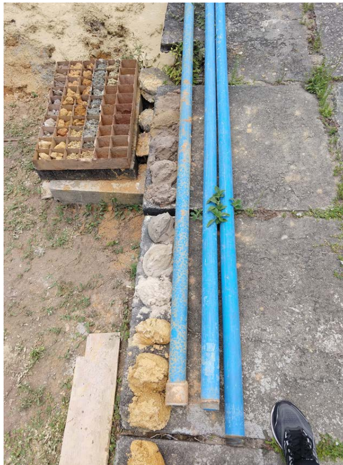
Figure 23. Drilling process – Soil samples and geomechanical tubes (source: SMART-Control project).
