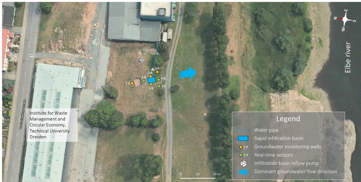
**Figure 3.** Detailed view of current system setup of the infiltration basin pilot site and the surrounding 5"-wells in Pirna, Germany
