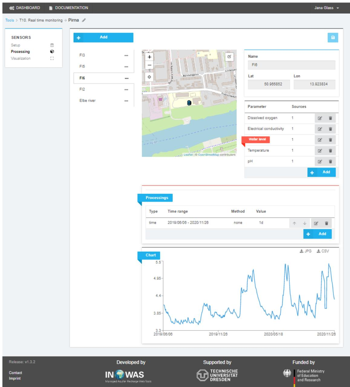
Figure 7. Screenshot of the time processing of sensor data on the web-based INOWAS platform
