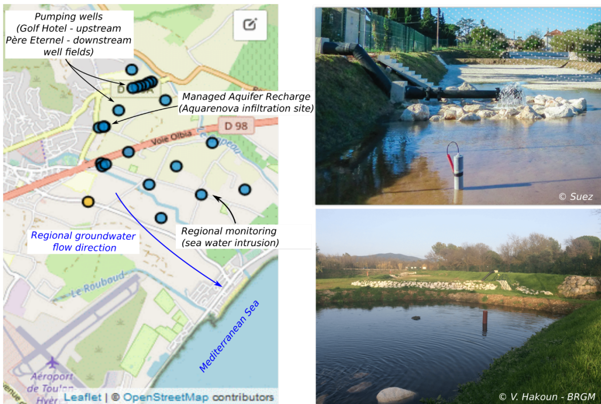
Figure 8: Map of monitoring sites and Managed Aquifer Recharge system in the Hyères les Palmiers site (France). Left : Notes the map give details about the multiscale monitoring network set up in the area. Right : Overview of the MAR system with recharge water filling the basin in the background and water level sensor casing on the foreground (top) and partially filled basin with water level sensor casing (bottom)
